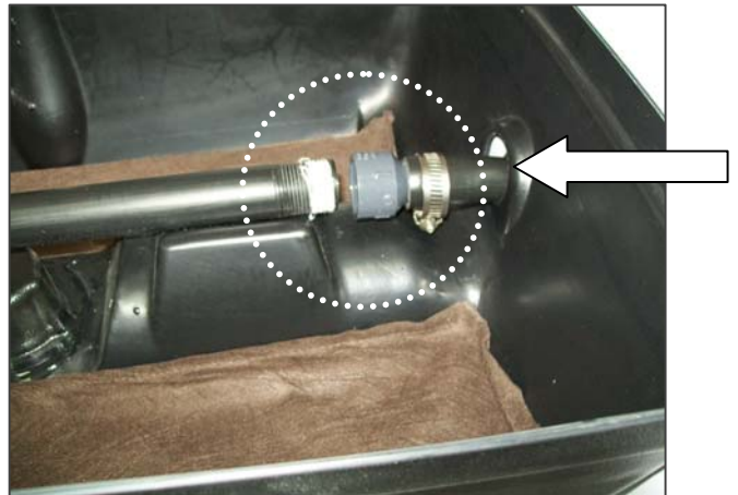
Figure 4.2 – Union femelle et bague de serrage / Clamps and female union
