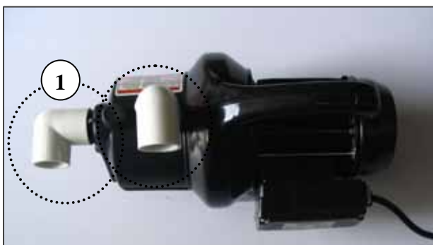
Figure 1.2 – Position des coudes (A2-03/2) 90 degree line elbow (A2-03/2)
